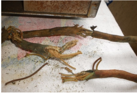
The status of the connecting cable between the receiver chassis and the speaker chassis.
