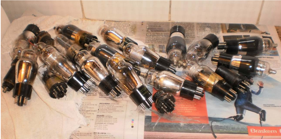
Thankfully, most valves, after testing, showed good emission.
