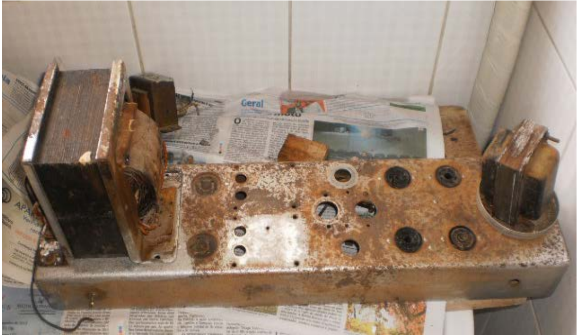
The rectifying chassis, output with dual push-pull and driver transformer.
