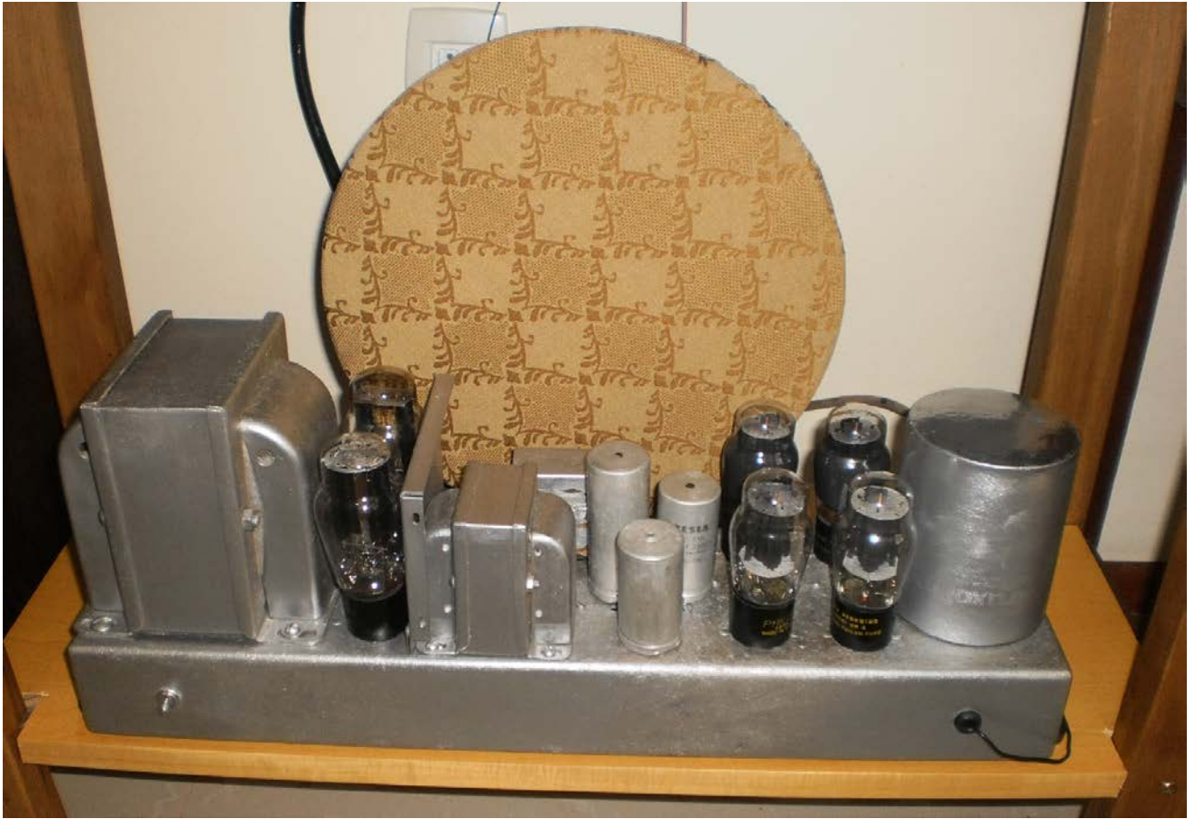
The rectifying chassis. Behind, the speaker set, output transformer and filter shock.
